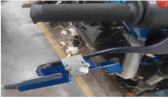
Figure 1: Clamping of load cell on brake lever
